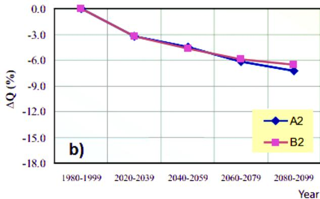
Fig. 5 Predicted change in (a) flood peak and (b) dry season's flow of the Red River (at Yen Bai station) relative to the period 1980-1999 based on climate change scenarios A2 (high CO<sub>2</sub> emission) and B2 (medium CO<sub>2</sub> emission) (source: [14])
