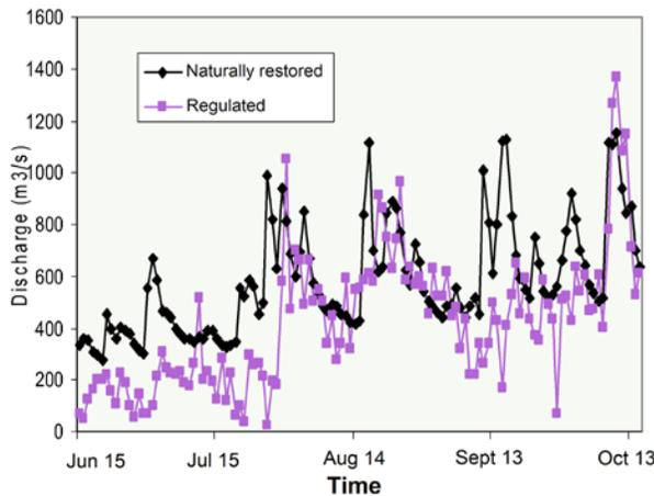
Fig. 3 Naturally restored daily flow and regulated daily flow in the Lixian River, 2010 (Source: [8])
