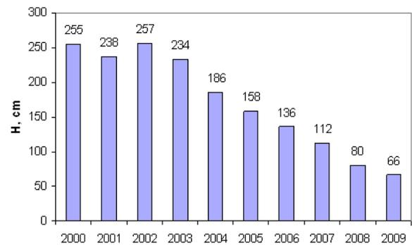
Fig. 4 The decline of minimum water level of the Red River at Hanoi station (source: [13])
